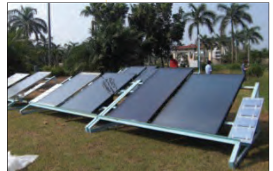
▲ Tropical test stand in Kochi, India with solar thermal collectors and components.
