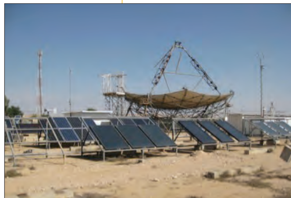
▲ Exposed solar thermal collectors in the Negev desert, Israel.
